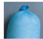
Socks filler expands and gels as liquid is absorbed
