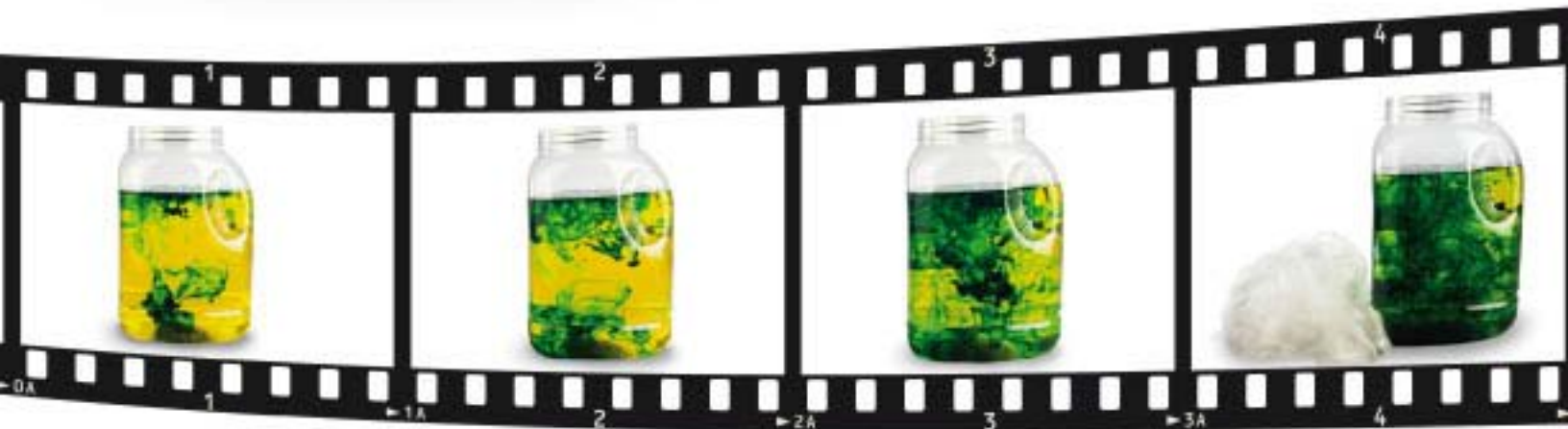
Above: The process that happens as an impurity is absorbed by the SpillLock™ fibers
